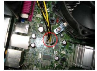
9. Disconnect P1 power cable and FDD data cable.
